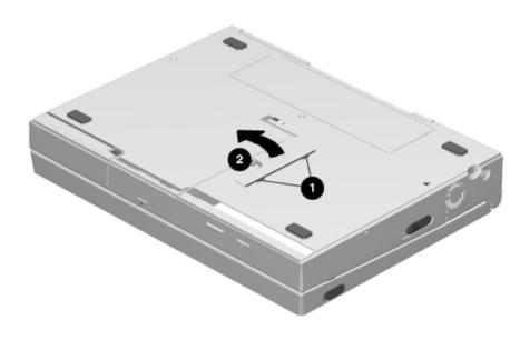
Figure 5-7. Removing the Auxiliary Battery Door
